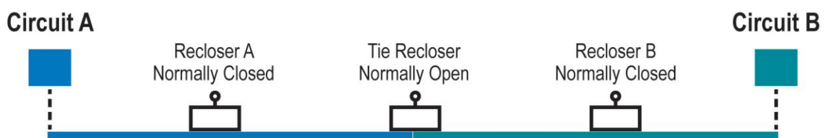
Exhibit 8.11.1 Typical Loop Scheme Diagram
