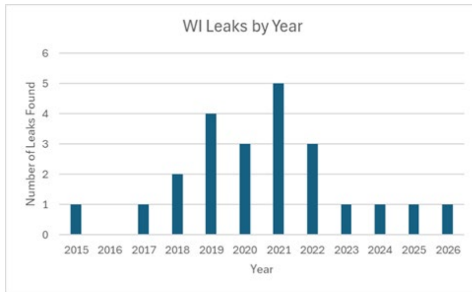
Figure 3: Wrought Iron Pipeline Leaks Found 2015 – 2024 and Projected 2025-2026
