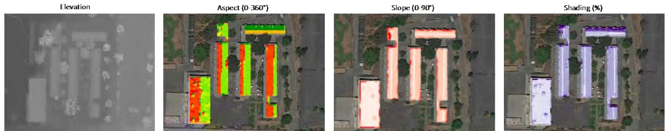
Figure 4. Elevation digital surface model and derived roof area characteristics used by the PV Rooftop model
