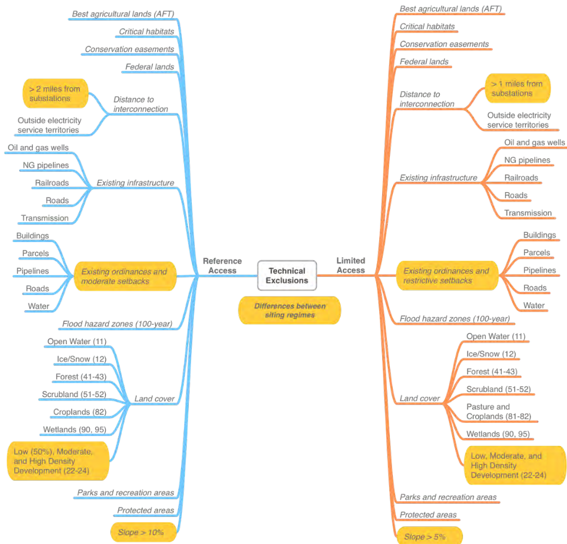
Figure 6. Ground-mount PV technical exclusions adapted from utility-scale solar siting regimes
