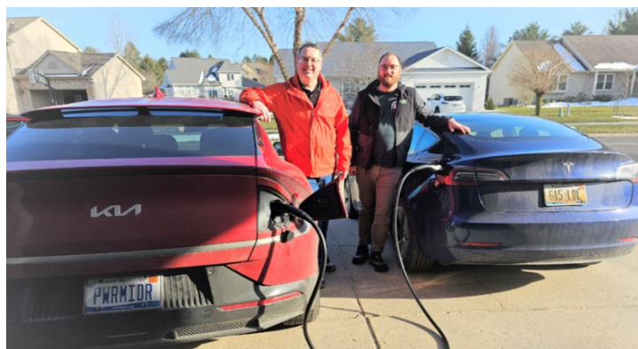
PowerMIDrive team members test a power-sharing residential L2 that utilizes a single NEMA 14-50 outlet – a solution that reduces customer costs and grid impacts of homes with multiple EVs
