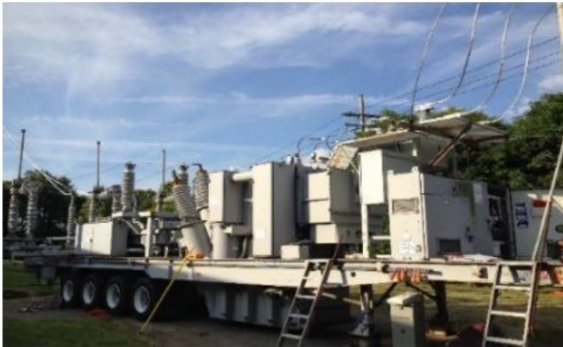
Figure 16. Portable Substation (left) & Mobile Generator (right)
