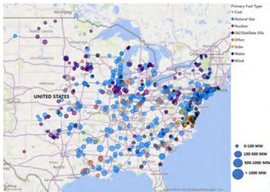
Figure 2: Location and Fuel Type of Unplanned Generation Outages and Derates During the Event (Bubble Size by MW for each Outage), as of December 24, 2022
