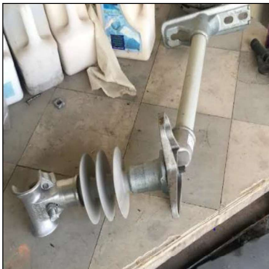
Single Phase Fiberglass Bracket with Insulator
