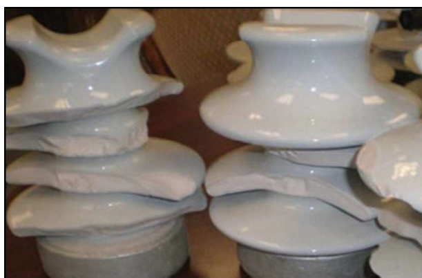
Defective Line-Post Insulator
