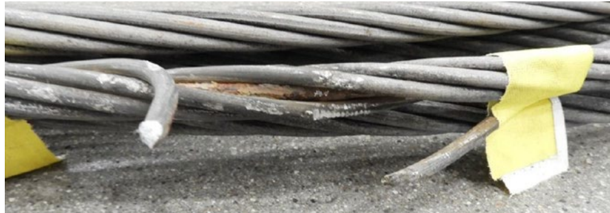
Figure 9: Existing Tie 4105 3/0 ACSR reduced tensile strength
