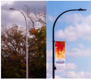
DTE Post Code 06: 28.75' black or silver single davit arm steel post mounted to concrete foundation-engineered to allow receptacles. Breakaway base option for this post design.
