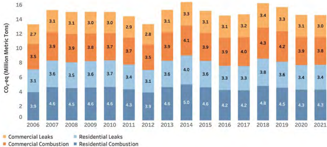
Figure 4-2: Residential and commercial sector CO 2 -equivalent emissions due to natural gas use in Maryland, with methane leaks evaluated at a 20-year global warming potential. The leak rate of 2.7 percent is calculated from Alvarez et al. 2018. 250
