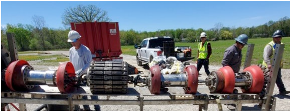
DTE Gas crew performing an ILI inspection – Figure 45
