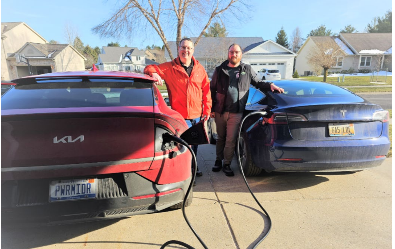
PowerMIDrive team members test a power-sharing residential L2 that utilizes a single NEMA 14-50 outlet – a solution that reduces customer costs and grid impacts of homes with multiple EVs
