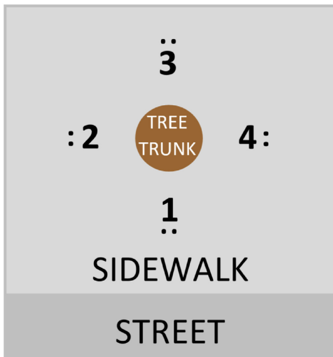
Fig. 1. Diagram of the protocol for sampling methane and oxygen concentrations in sidewalk tree pits. The black dots represent the two adjacent holes, one for the methane sample and one of oxygen sample, that were created at each of the four locations around the tree trunk.
