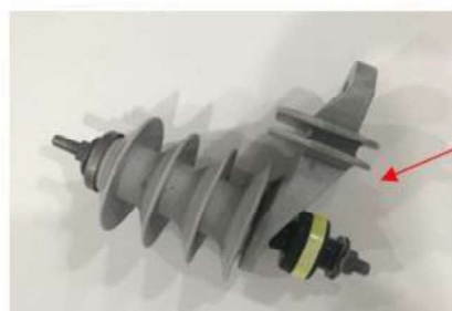
Side View of Arrester
