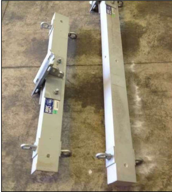
Acceptable Fiberglass Cross-arm
